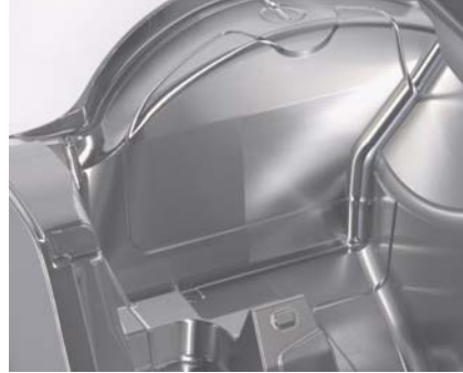
Surface finishes obtained by using FF/CAM can drastically reduce, and in many cases eliminate costly bench work.
